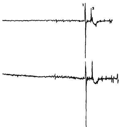
Fig. 8. Replicate separations of human hemoglobin. 1 = Methemoglobin; 2 = oxyhemoglobin. Capillary, 12 cm \times 20 \mu m I.D.; protein concentration, 0.3 mg/ml.
